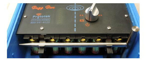
All operations are controlled by the single knob. The positions are clearly marked, and correspond to "Off", Battery Check, and 4 transmitter frequencies. Whenever the BuzzBox is on, it beeps once per second. In the Battery Check position the line of green LEDs to the left of the knob tell you the condition of the batteries. When they are fresh,
