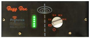
In use, select any of the 4 transmitter frequencies with the knob. If you have the cables unplugged for Inductive locating, the LEDs that indicate signal strength will be **green**, and they will light sequentially from the bottom to the
