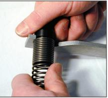
Next, place the wrench under the spring and hook the single tooth of the wrench onto the tail end of the spring. Let the curve of the spring nest into the curve of the wrench.
