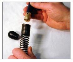
Place the transmitter into the carrier, metal end first. Be sure your battery has been placed in the transmitter correctly as well - the positive end of the battery goes in first.
