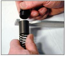
Grip the Spring Carrier in one hand and push down while the wrench is still engaged. With your other hand, open the plug end of the carrier by turning it toward you (counter-clockwise).
