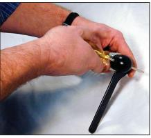
For **Spring Carrier 1.7**, put a 1/4" or smaller round shafted screwdriver or other tool through the hole in the plug end to turn it.
