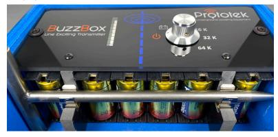
All operations are controlled by the single knob. The positions are clearly marked, and correspond to "Off" U Battery Check and 4 transmitter frequencies. Whenever the BuzzBox is on, it beeps once per second. In the Battery Check position the line of green LEDs to the left of the knob tell you the condition of the batteries. When they are fresh, all 8 LEDs are lit.
