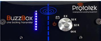
When the cables are plugged in and connected for Conductive locating, the number of lit blue LEDs indicates the quality of the ground in your setup. You should endeavor to cause as many LEDs to light as possible by wetting the ground around the rod or choosing an alternative ground method.
